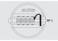
2. While the Master Key remains in this position, carefully pull off the number wheel housing to the left.
