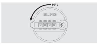
2. Turn the number wheels to lock the lock. In this state the release button cannot be pressed and the lock cannot be unlocked.
