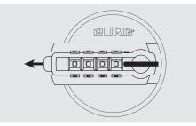
3. Insert a pin on the back of the number wheel housing as far as possible into the first opening from the left. Turn the number wheel from the front until it engages. Repeat the procedure for all number wheels. Once all the number wheels have engaged, the valid code can be read off.
