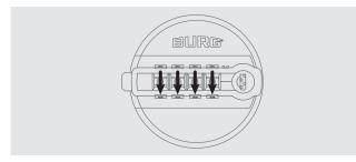
2. Press the release button and hold it. Turn the lock 90° to the right. The lock is now unlocked.
