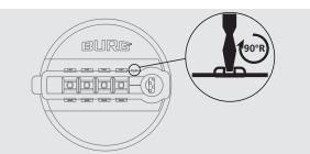
2. Carefully turn the number wheels one after the other until they engage (from top to bottom / from left to right). Do not move to the next number wheel until the previous number wheel has engaged. When all number wheels have engaged, the valid code can be read off.
