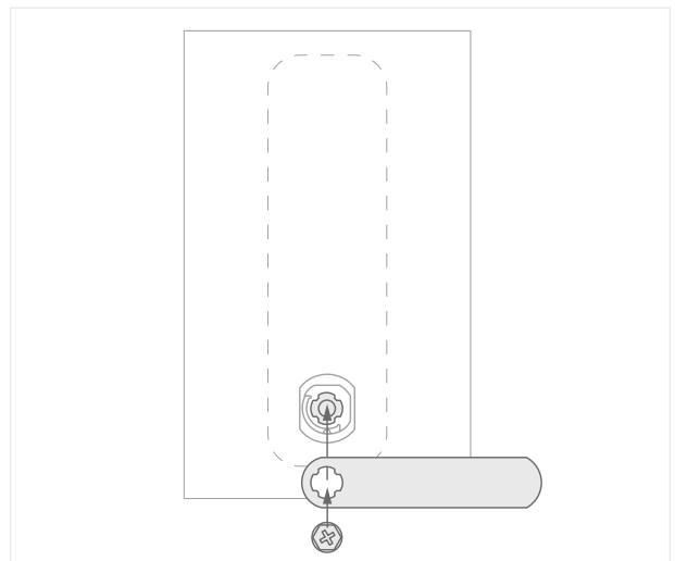
5 Then check whether the cam has sufficient hold on the striking plate or the rebate when closed. It should be possible to turn the cam to its end position without pressure or resistance when locking the locking system.
