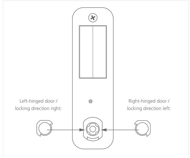
4 Fit the cam and tighten it hand-tight using the enclosed cam fixing screw and a Phillips screwdriver (e.g. size PH 2).
