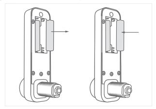
Replace the rubber seal. Refit the locking system with the nut and screw (see page **8** "Assembly").
