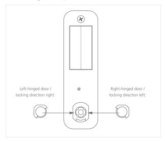
4 Fit the cam and tighten it hand-tight using the enclosed cam fixing screw and a Phillips screwdriver (e.g. size PH 2).
