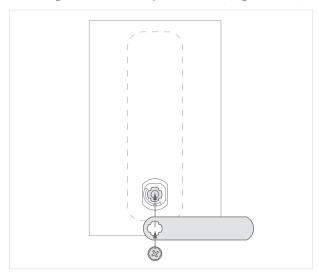
5 Then check whether the cam has sufficient hold on the striking plate or the rebate when closed. It should be possible to turn the cam to its end position without pressure or resistance when locking the locking system.
